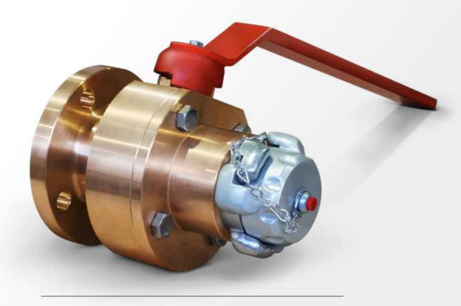
A ball valve is a quarter turn shut-off valve that controls the flow of fluids by a rotary ball. The spherical rotary ball consists of a straight bore through it. The pipe is in the open position when the bore is aligned in the same direction as the flow, allowing the fluid to pass through it. When the bore is rotated 90 degree from the flow path, the valve is closed, and the flow is blocked. Ball valves are used for its reliable sealing properties and long service life.
