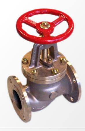
Due to their configuration, FHT bronze globe valves are perfect for regulating or limiting fluid. Depending on system needs, design or position, they could generate different load losses on the line. Globe valves are multiturn, in which the obturator is achieved by means of a disc or plug that cuts the passage of fluid in a seat that is usually parallel to the circulation in the pipe.
