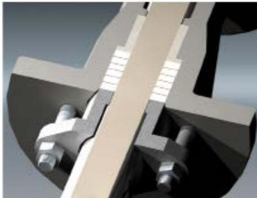
Packing rings are tightened with the stuffing-box gland to give a radial seal to atmosphere around the ram.
