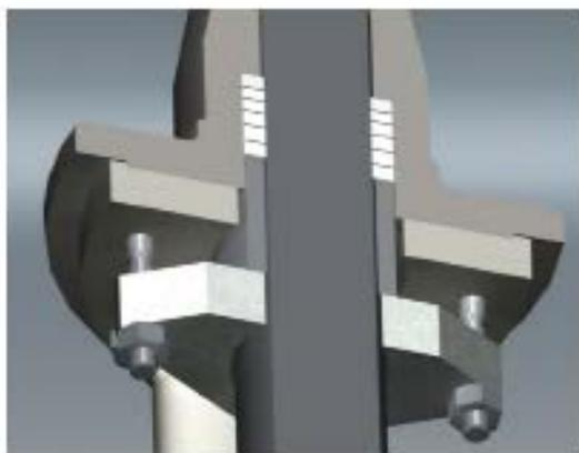
Ram-Seal<sup>®</sup> valves use packing rings for sealing to atmosphere. The packing rings are tightened using the stuffing-box gland to give a radial seal to atmosphere around the ram. Packing rings can be ordered in TVE/KEV or Graphite (suitable for high temperature or FIRE SAFE operation) or even in a mix of both. More specialized packing arrangements are available, including Chevron PTFE or Garlock graphite sealing sets.
