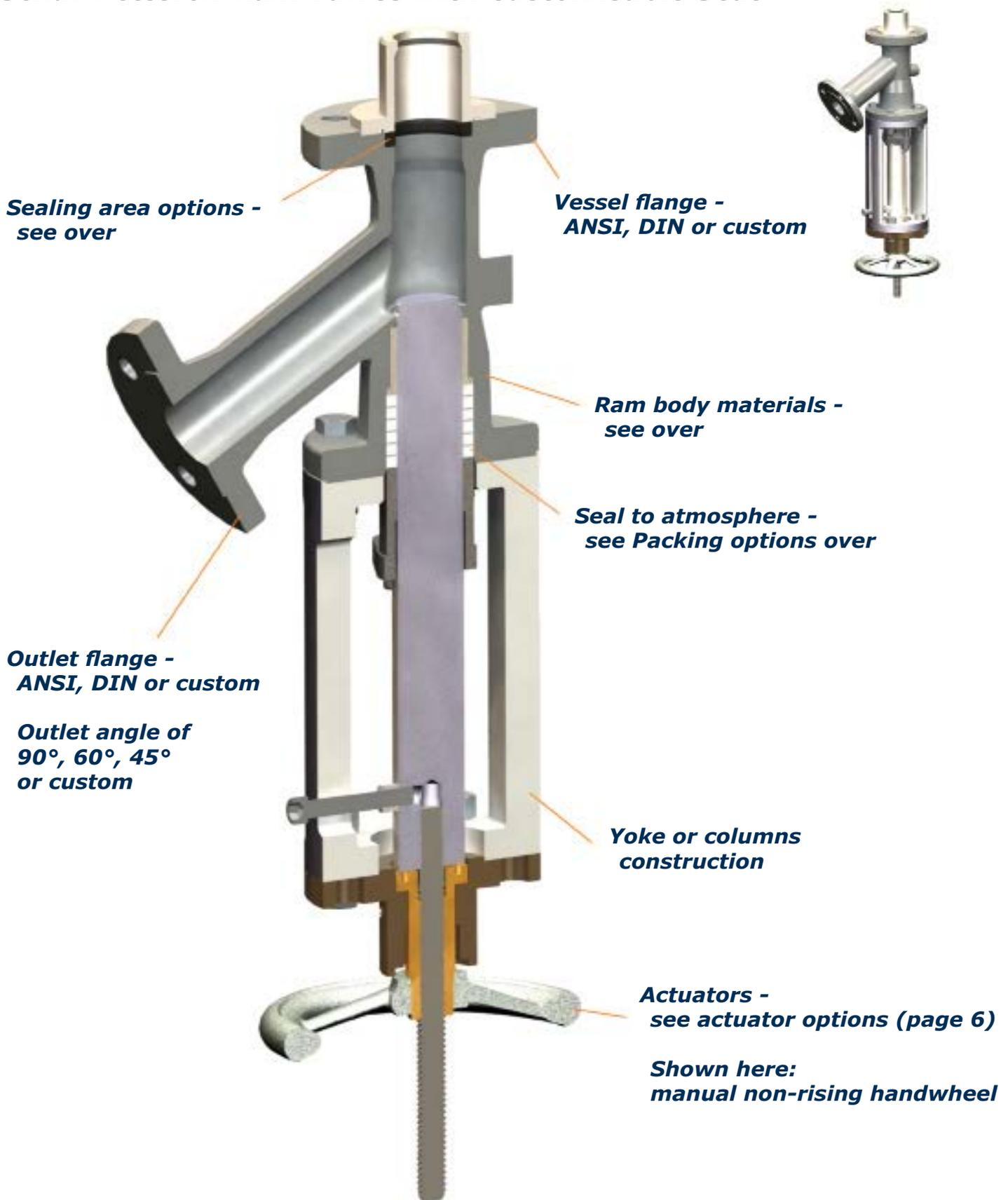
**Ram Valves are used when full flow is essential to drain reactors and vessels, flush pipelines, inject media such as kill gases and catalysts and take large samples.**
