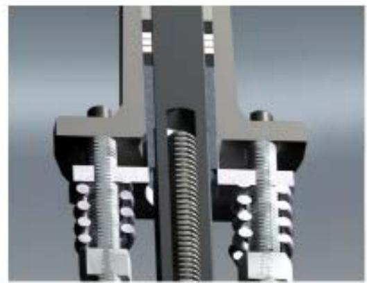
Rod-Seal<sup>®</sup> valves offer the unique Super Closure feature. A cross-head component, mounted at the end of the ram, compresses the stuffing-box gland only when the valve is fully closed. Thus, all the forces of actuation are carried by the guide bush to the packing rings and the radial seal at the top of the valve. This increased closing power ensures a tight shut-off to the process and the atmosphere. This sealing force eases when opening the valve.
