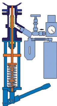
The 32PH has a metal bellows seal for zero leakage to the atmosphere. Options include leak detection chambers and venting canisters.
